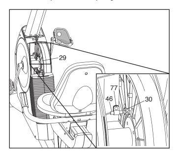
Then, retighten the M4 x 16mm Screw (77). Plug in the power adapter and turn the Pulley (29) for a moment. Repeat these actions until the console displays correct feedback.
